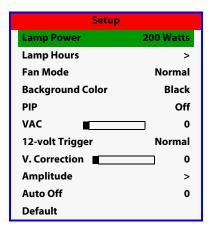
**VAC:** Use the VAC control to increase or decrease the V<sup>2</sup> Aperture Control setting. VAC lets you control the aperture or iris size (the physical opening through the lens; similar to an "f-stop" on a camera). Doing so allows you to optimize brightness and contrast according to the amount of ambient light in the viewing area.
